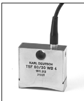
Line focused PVDF-probes with z = 20, 40, 60, 85 and 110 mm
