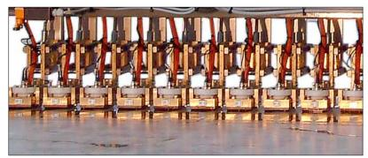
Probe holders for the strip middle: Hardened skids guide the gimble-mounted probes along the strip surface.
