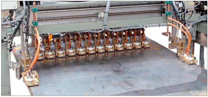
Narrow strips are fed through the inspection system in a centric manner. Only the probes above the strip are then active. The individual probe holders are pneumatically lowered into the test position. The end of the strip or largely damaged zones within the strip are automatically detected and the probes are lifted into the satefy position.
