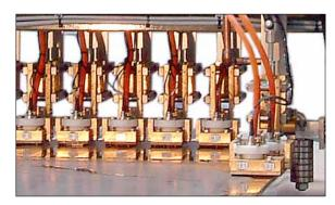
The strip edges are separately inspected with a test trace between 25 mm and 50 mm. Rollers which are pneumatically guided along the strip edge allow a precise positioning of the probes. 100% of the strip edge is covered.
