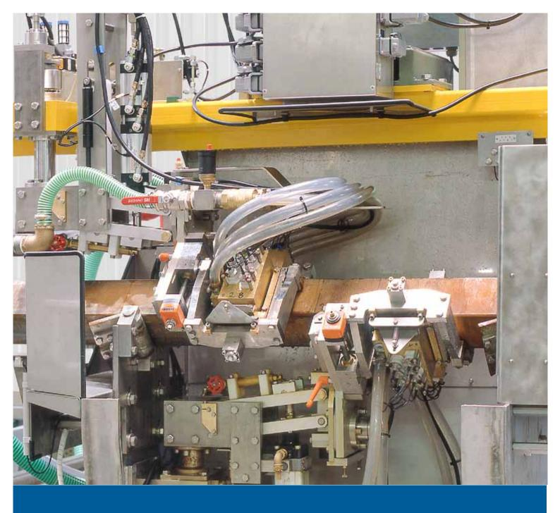
ECHOGRAPH-KNPS Ultrasonic Inspection of Billets
