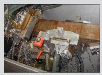
Four probe holders for quadratic billets, each carrier with seven probes and positioning from all four sides. The guidance is achieved by guiding rollers and hard-metal skids.
