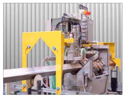
ECHOGRAPH-KNPS billet testing system Light barriers check the billet position.
