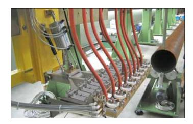
Inspection of tubes with longitudinal weld (ERW tubes):
