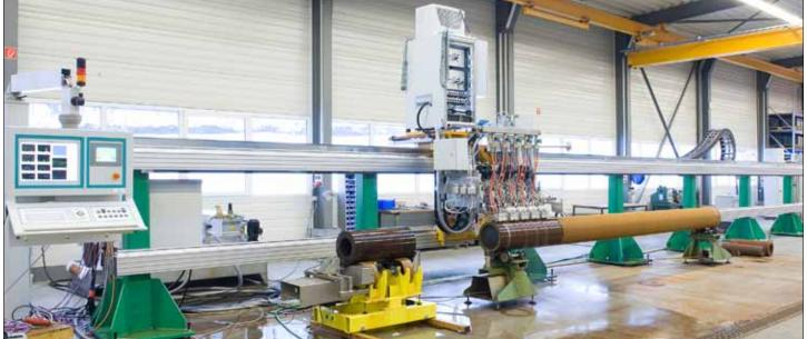
Tube testing portal during assembly at KARL DEUTSCH system's workshop. A provisional calibration stand (yellow) is used for the sensitivity adjustment of all probes by means of a short tube segment. The probe holders are currently placed onto a production tube. This system was designed for a maximum tube length of 12 m. A modern phased array testing electronics with 192 parallel electronic channels was employed for an electronic beam angle adjustment and overlapping sound beams.
