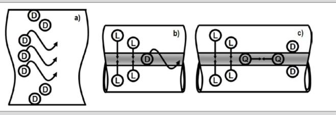
Typical testing tasks for the ERW-pipe inspection.
