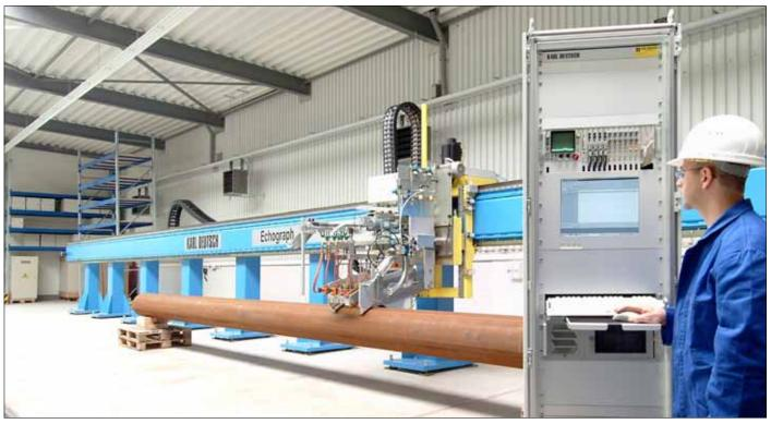
Testing portal (offline testing machine) during assembly at KARL DEUTSCH workshop
