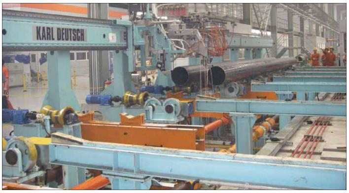
Testing Portal (Offline Testing Machine): Onsite operation with transverse conveyor for pipe feeding and linear discharging of the pipes. This machine was also equipped with two additional probe holders for the pipe end inspection.
