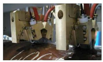
Probe holders with angular incidence for the detection of longitudinal defects. Stable ultrasonic coupling is achieved by water jet coupling (also called squirter technique). The incidence angle can be adjusted without steps for a perfect setting with respect to pipe diameter and wall thickness and without changing the probe.
