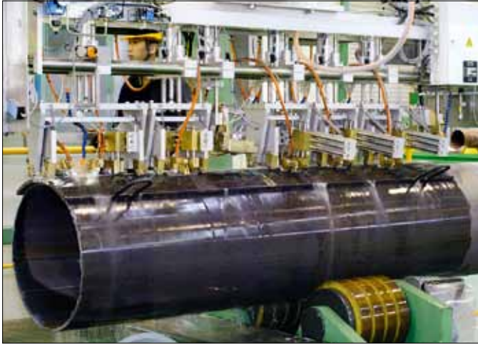
Probe holders of weld testing system on pipe segment for system calibration (photo with courtesy of EEW-Korea).
