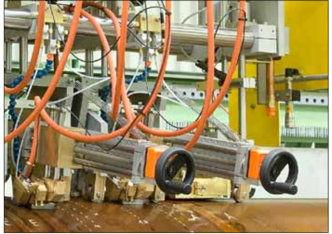
Probe holders for the detection of longitudinal defects: Spindles with position gauges are used to adjust the distance between the probes and the weld seam.
