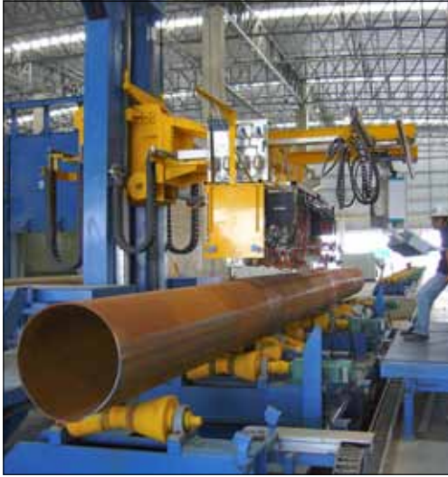
The testing mechanics with the probe holders is mounted to a stable machine stand. The ultrasonic probes are positioned near the weld seam in the 12 o'clock position and symmetrically to the weld seam. The height of the horizontal boom (in yellow) and the ultrasonic probes are pre-positioned in accordance with the pipe diameter.
